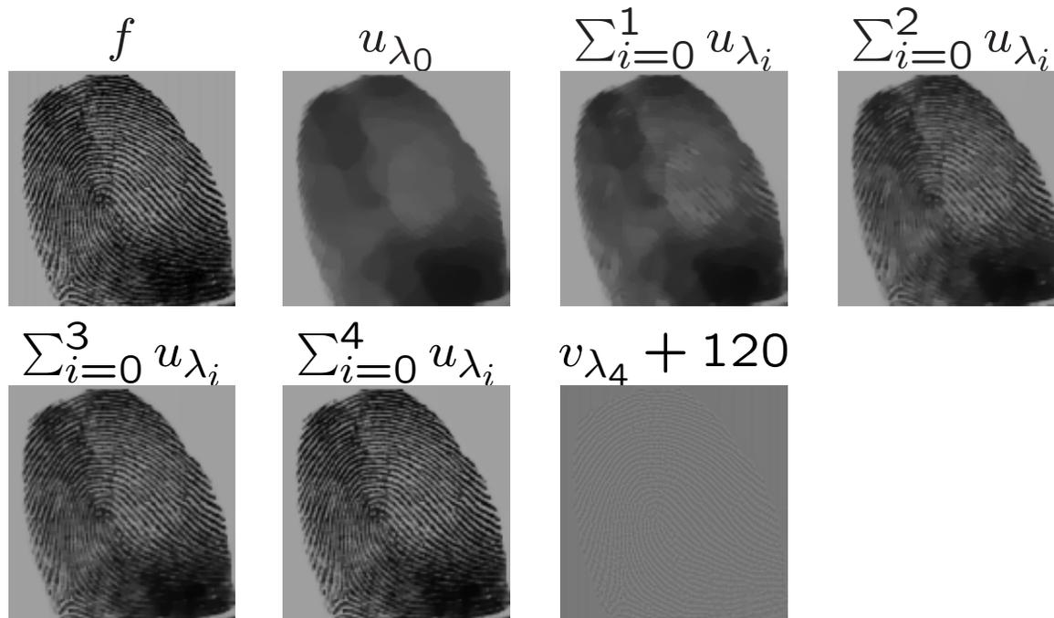
Decomposition of an initial image of a fingerprint for 5 steps with  $\lambda_0 = .01$ .
